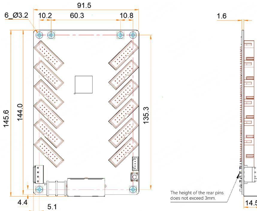
Tolerance:  $\pm 0.3$  Unit: mm
